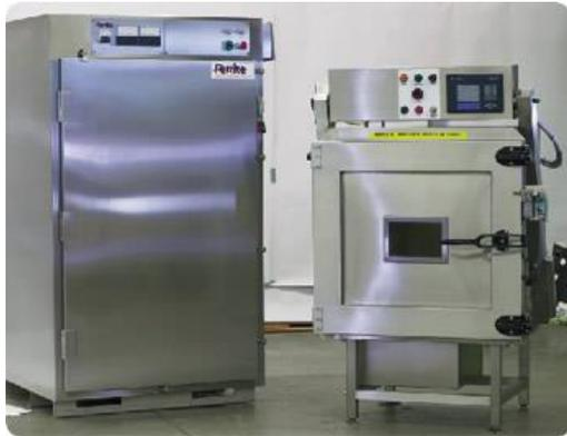
The microwave energy is then transmitted to a cavity of varying type for application to the material being treated. For example, pictured left is a small batch tempering system FMT produces, the MIP-4. Included in the photo is a standard 75 kW GET2024 generator.
